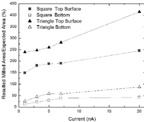
**Figure 5.** Relationship between the surface areas of the square patterns and triangle patterns per each current value, where the top surface area indicates the milled area of diamond surface, and the bottom surface area indicates the milled area at the bottom of the trench.
