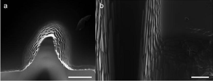
**Figure 4.** Nano-terraces on the sidewalls of milled single-crystal diamond (ion beam current of 20 nA). a) Top view of the 150  $\mu\text{m}$ -depth hole in Figure 2 (right trench); b) Side view of the intersection of trenches A and B in Figure 1. Scale bars represent 3  $\mu\text{m}$  in *a* and 1  $\mu\text{m}$  in *b*.
