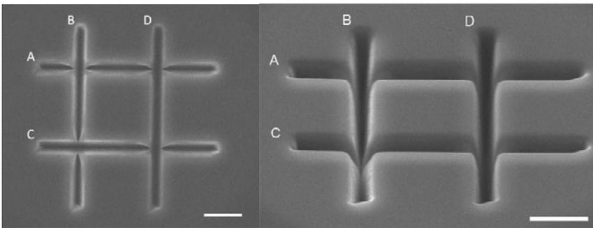
**Figure 1.** The linear patterns were etched sequentially, starting with line A(from left to right) at 1  $\mu\text{m}$  x 50  $\mu\text{m}$  x 50  $\mu\text{m}$ ; then line B(from top to bottom), C(from left to right), and D(from top to bottom), with identical dimensions. The scale bars in both Figures represent 10  $\mu\text{m}$ .
