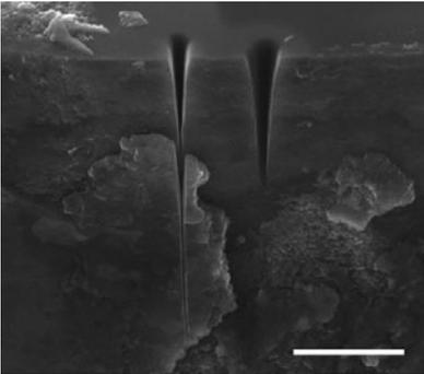
**Figure 2.** The trench in the left was designated a depth of 50  $\mu\text{m}$  (actual depth was 12.3  $\mu\text{m}$ ), and width of 1  $\mu\text{m}$  (actual width was 4.1  $\mu\text{m}$ ). The second trench in the right was set for a depth of 150  $\mu\text{m}$  (actual depth was 13.5  $\mu\text{m}$ ), and a width of 1  $\mu\text{m}$  (actual width was 6.3  $\mu\text{m}$ ). The scale bar represents 20  $\mu\text{m}$  in length.
